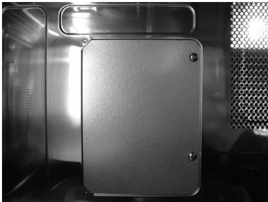
Figure B.1. Microwave oven waveguide cover where the microwave energy enters the oven interior. Photo by the author, 2011.
