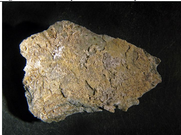
Figure 6: This 2 inch sawed slab has over two hundred 0.1 to 0.5 mm orange anatase crystals.
