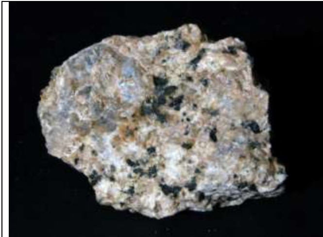
Figure 6 Anorthite-Labradorite 5 cm specimen. The black amphibole is likely augite. Piper Mtn. Gilford, NH
