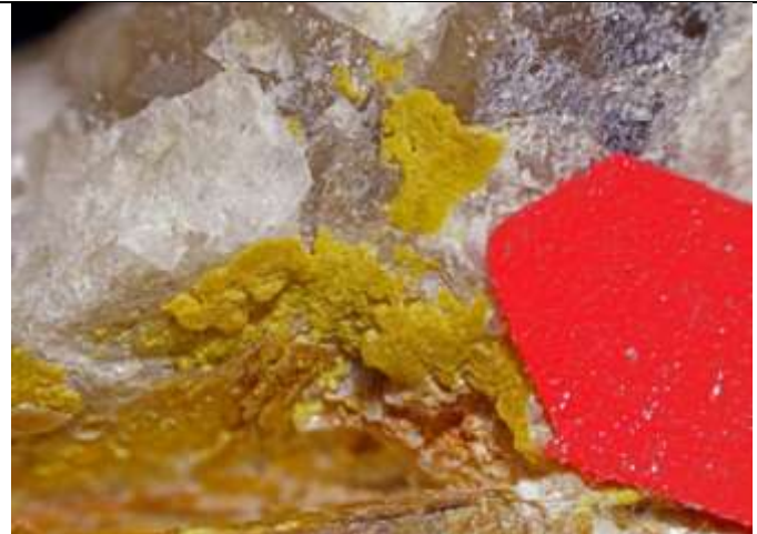
HUMBOLDTINE Government Pit, Albany, NH 7.5 mm FOV. Red arrow points to EDS grain sample point
